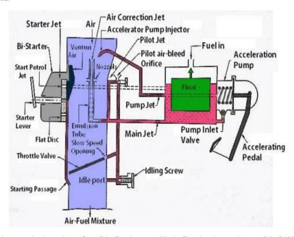
A float with a tapered valve at the top face of the float is arranged in the float chamber to take care of the fuel level in it as shown in the below schematic representation.
